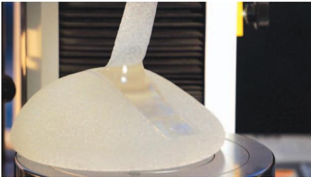
**Fig. 9.** Gel/shell failure of the Mentor CPG.
