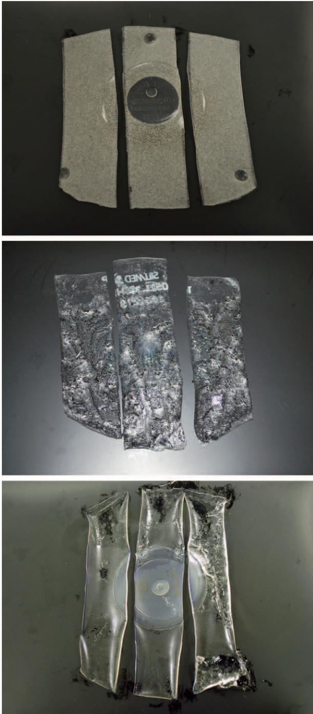
**Fig. 3.** Images of 3 types of peel test failures: gel/shell failure (*above*), gel/shell integration (*center*), and mixed gel/shell failure and integration (*below*).
